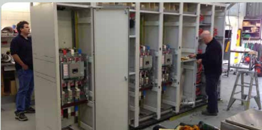
Figure 2: Forth pump station electrical switchboard in construction
