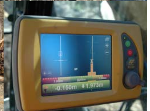
The excavators digging the pipeline channel were GPS-controlled (lower right) from a base station (lower left).
